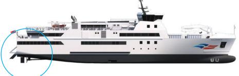
We have been working closely with Piriou developing and finalising the vessel designs ready for building to commence in June. The Scillonian IV design progression has seen the introduction of a Hull Vane®.
